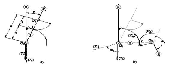
Fig. 3a. The mechanism of a scissor and its geometrical parameters
