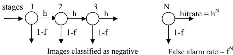
Figure 1. Cascade classifier with N stages [3]
