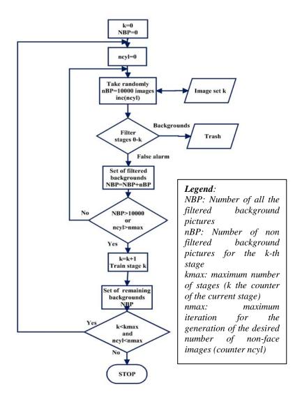
Figure. 2. Significant background generator
