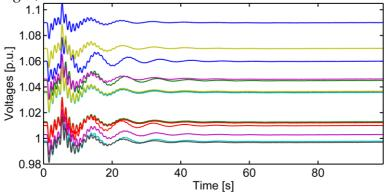
Fig. 8 Normal operation with load variations
