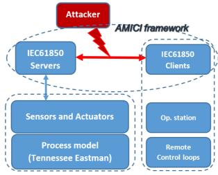
Fig. 2 AMICI extended with IEC 61850
