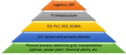
Fig. 1 Hierarchical structure of modern CI
