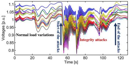
Fig. 9 Effects of integrity attacks on bus voltages
