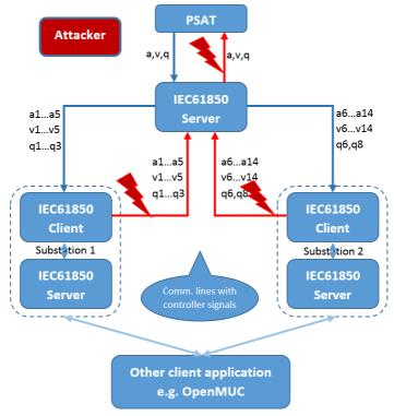
Fig. 3 The framework combining PSAT and IEC 61850
