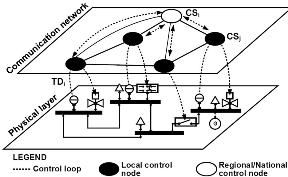
**Figure 1:** Architecture of modern Networked Critical Infrastructures.
