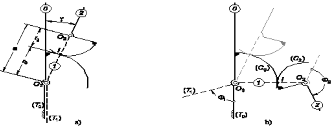
Fig. 3a. The mechanism of a scissor and its geometrical parameters
