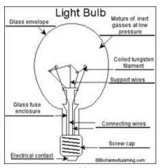
Figure 4: Example of diagram. Source: <a href="http://www.nomenclaturo.com/electric-electricity">http://www.nomenclaturo.com/electric-electricity</a>
