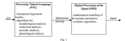
The synthesizer is based on two important modules, namely: the Natural Language Processing Module (PNL) and the one for the Digital Processing of the Signal (PDS), as can be seen in Fig. 1. Next, we shall present the principles on which the formalization of the Romanian language phonology is based, in order to realize the phonological transcription of a written text, a transcription capable, in the end, to reproduce the sound units (diphonemes) in a word, along with prosodic information.
