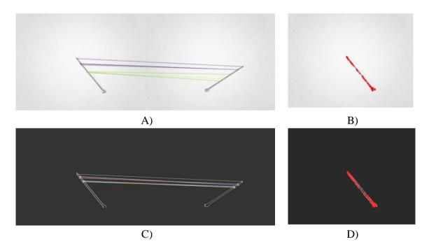
**Fig. 3.** Example for the processing realized by the similarities finding algorithm for a thin shape. A) Filtered feature comparison on original image; B) Features from original image; C) Filtered feature comparison on exterior contour; D) Features from exterior contour.
