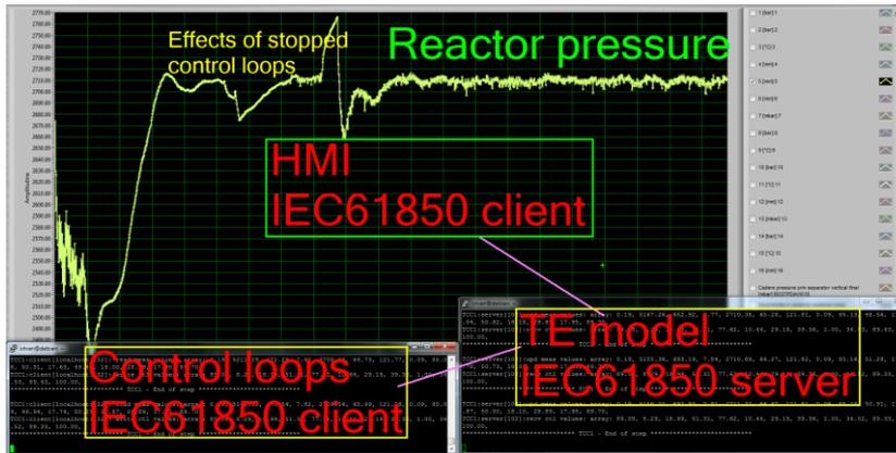
Fig. 5 Experimentation view – attacks that disturb control loops' operation
