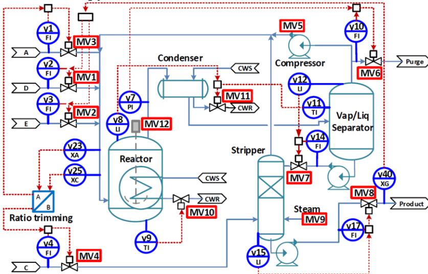
Fig. 4 The Tennessee Eastman chemical process instrumentation diagram
