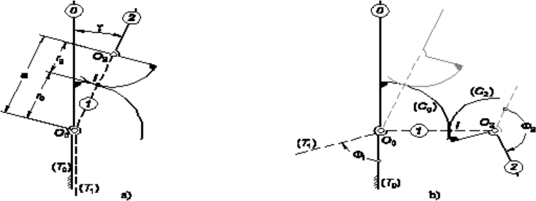
Fig. 3a. The mechanism of a scissor and its geometrical parameters
