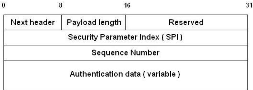
Figure 3.1 – AH header
