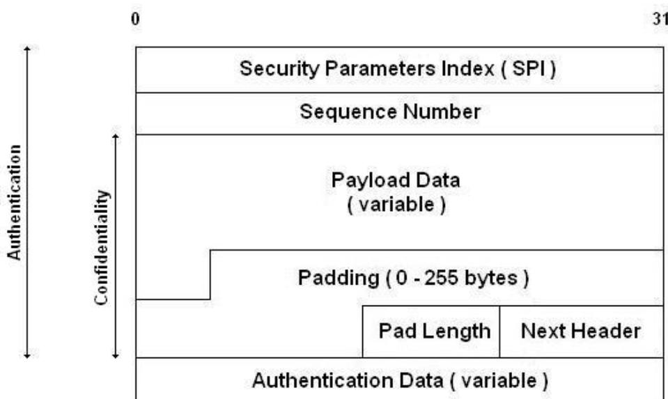
Figure 4.1 – ESP packet
