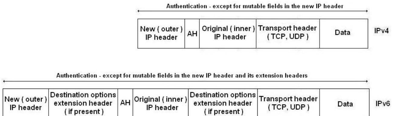
Figure 3.3 – AH tunnel mode
