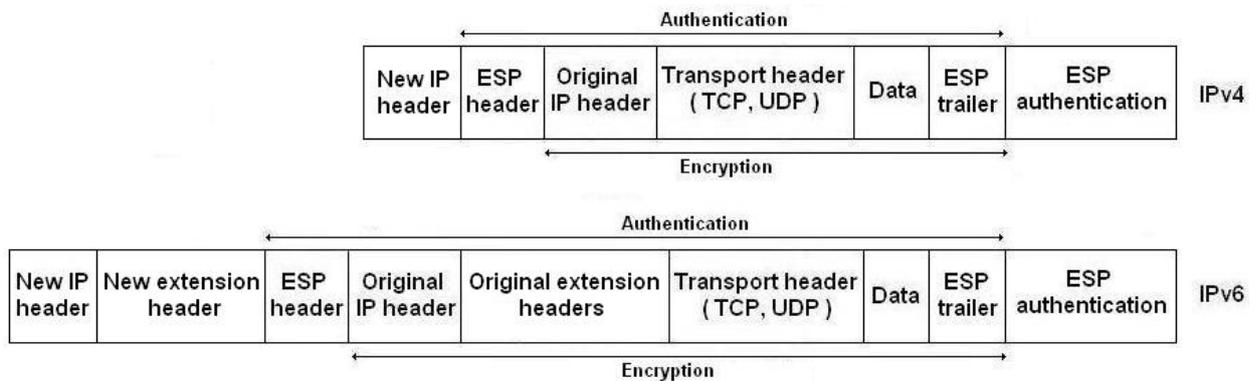
Figure 4.3 – ESP tunnel mode
