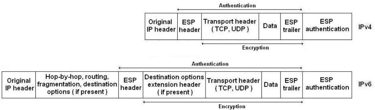
Figure 4.2 – ESP transport mode
