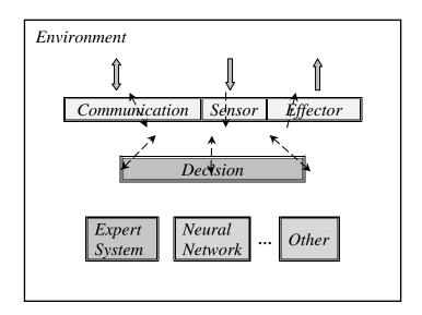
**Figure 1.** The hybrid expert system agent architecture
